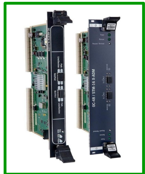
COST-EFFECTIVE 2-PORT OC-48/STM-16 X-ADM MODULE FOR THE NIMBRA ONE AND 300 SERIES
